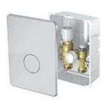
The IC Box is a regulation unit for individual underfloor heating circuits that can be connected directly to the existing return installation and does not require an additional heating pump or mixing valve. It also features a thermostatic head for direct mounting or with remote sensor, including an integrated manual vent valve and installation housing for flush mounting.
