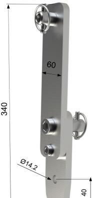
If the GEROtherm® weight connector is mounted directly on the 20 kg additional weight, the probe is perfectly centred. A spring cotter pin supplied with the additional weight is used to secure the connection.
